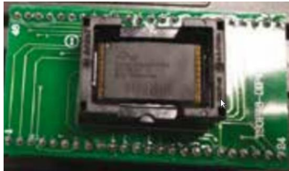
Figure 5. Example of a TSOP package flash to be read using an adapted socket and a programmer
