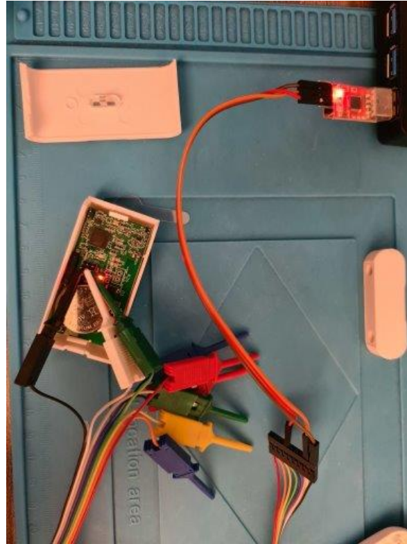
Figure 4. Interfacing with the UART of a magnetic door LoRaWAN sensor
